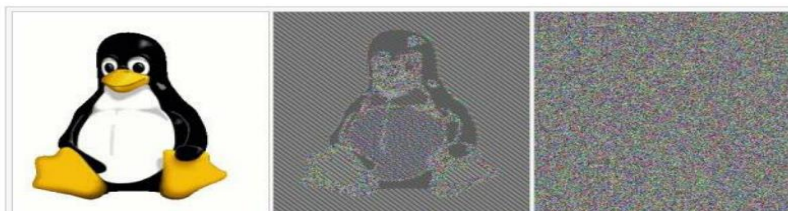
Original image Encrypted using ECB mode Modes other than ECB result in pseudo-randomness
